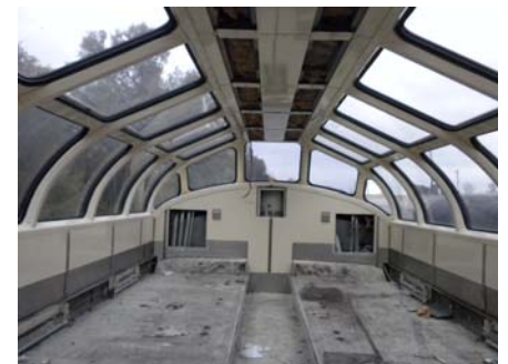
New Dome Glazing & Interior Paint
