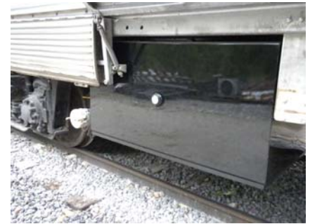
New holding Tank
